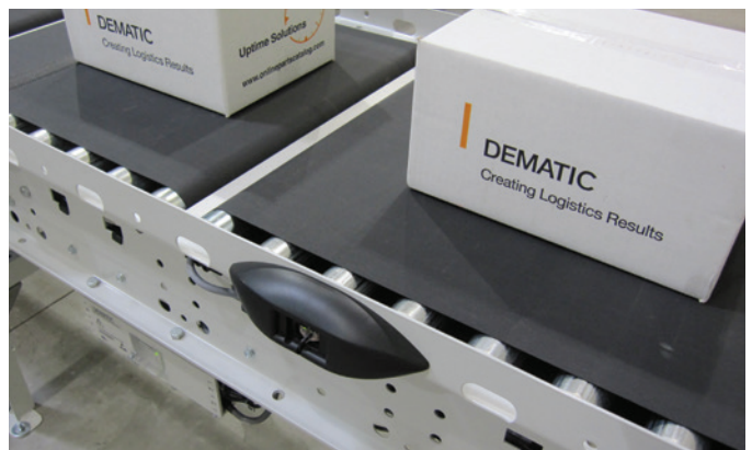
Cover on side channel protects electronic sensor
